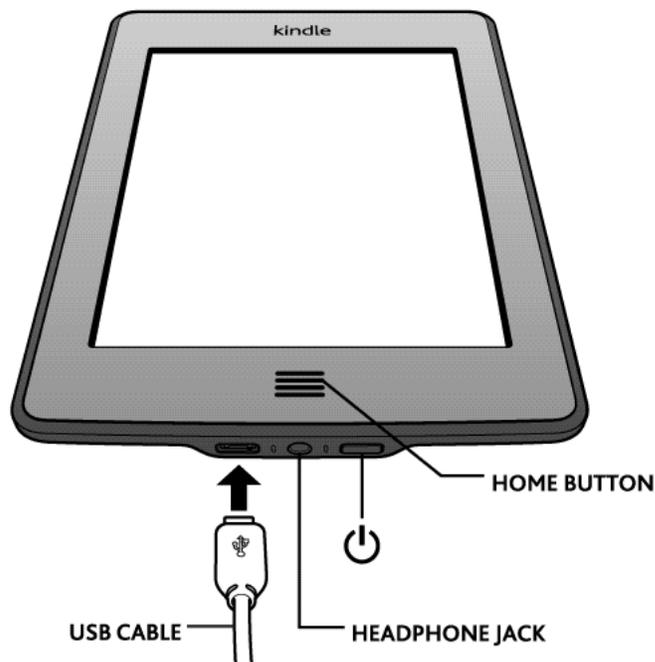
Below the screen is the Home button. At the bottom edge of the Kindle are a headphone jack, charge indicator light, power button, and micro-USB/power port. On the lower back are two speakers.
